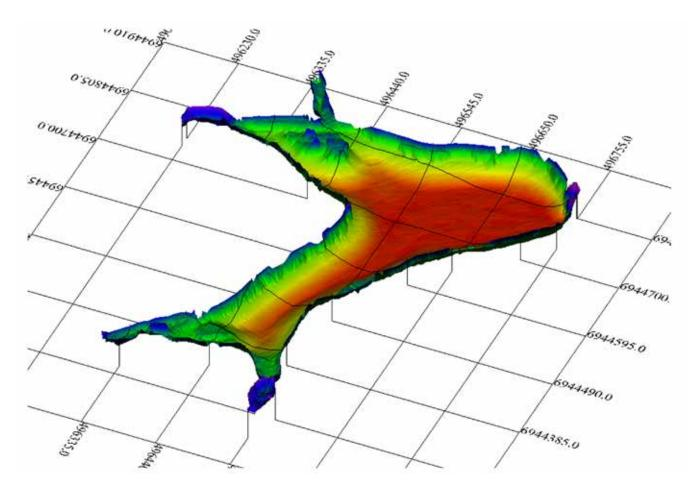
Figure 15. 3D Sludge Surface Elevation.
