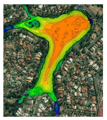
Figure 14. Sediment Surface Elevation.
