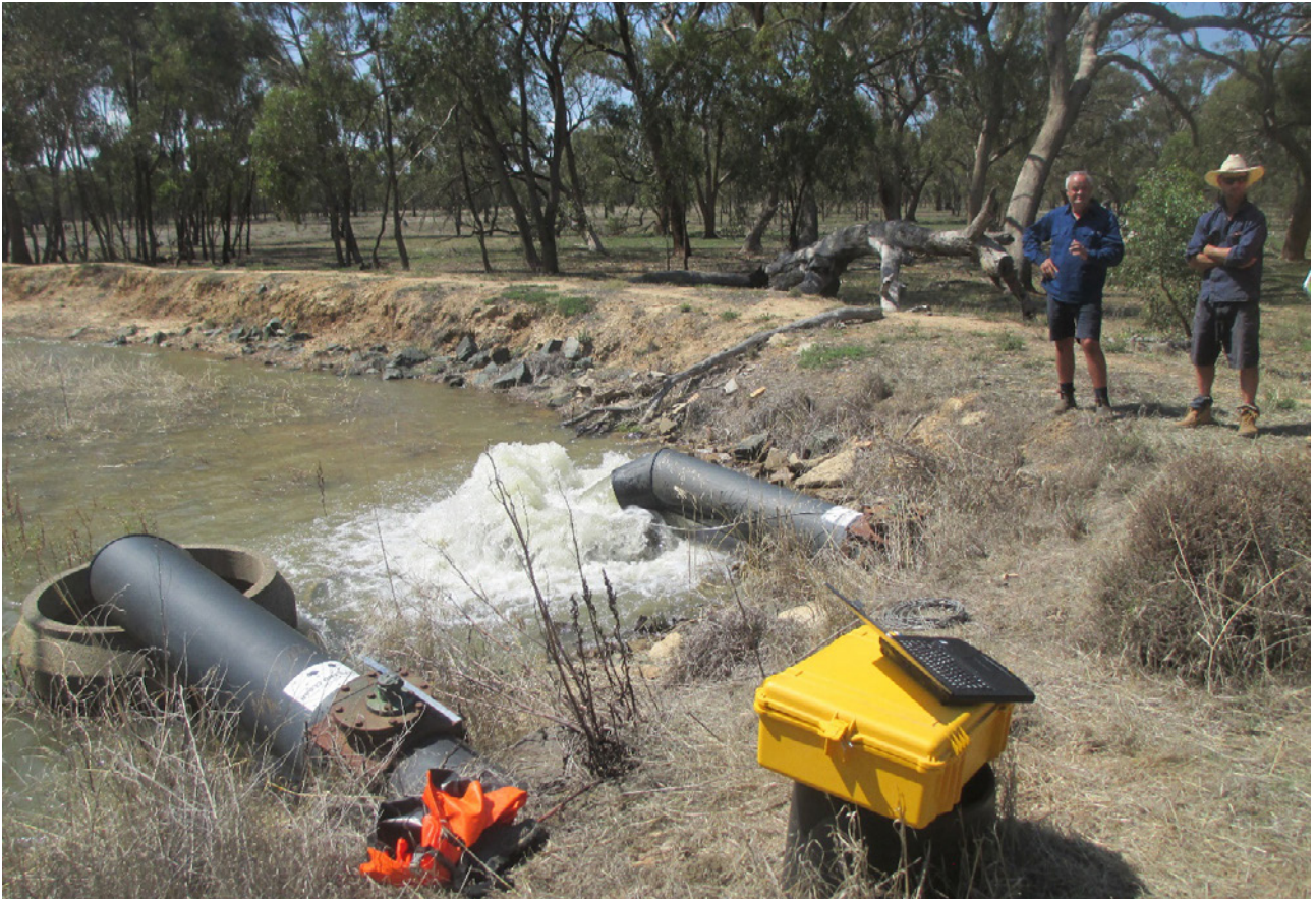
Multi-Beam Doppler (end of pipe)
