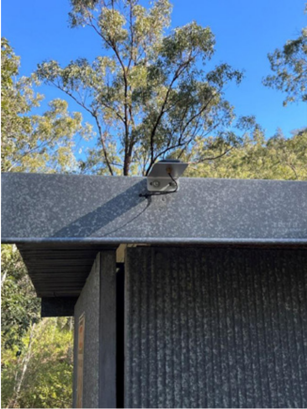
Eungella Dam TW - 15minute data, 1 hour transmission, with EWS Switch (Iridium telemetry unit and datalogger)
