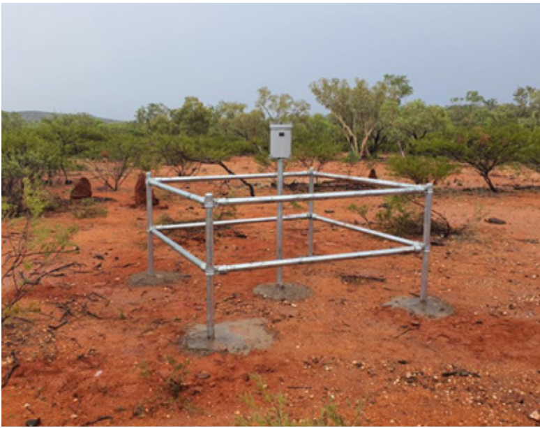
Lake Julius Upper Catchment Rain Gauge with Ontoto Pulsar Satellite Modem
