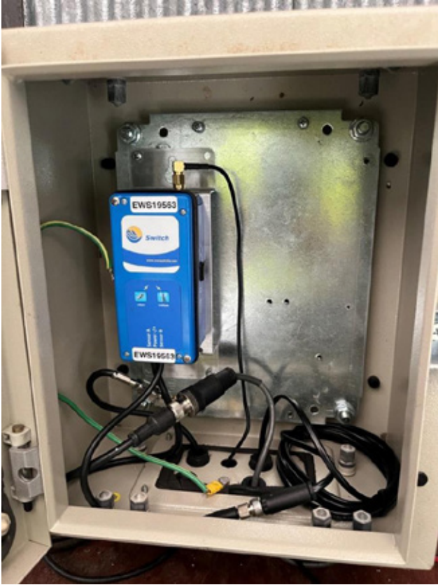
Eungella Dam TW - 15minute data, 1 hour transmission, with EWS Switch (Iridium telemetry unit and datalogger)
