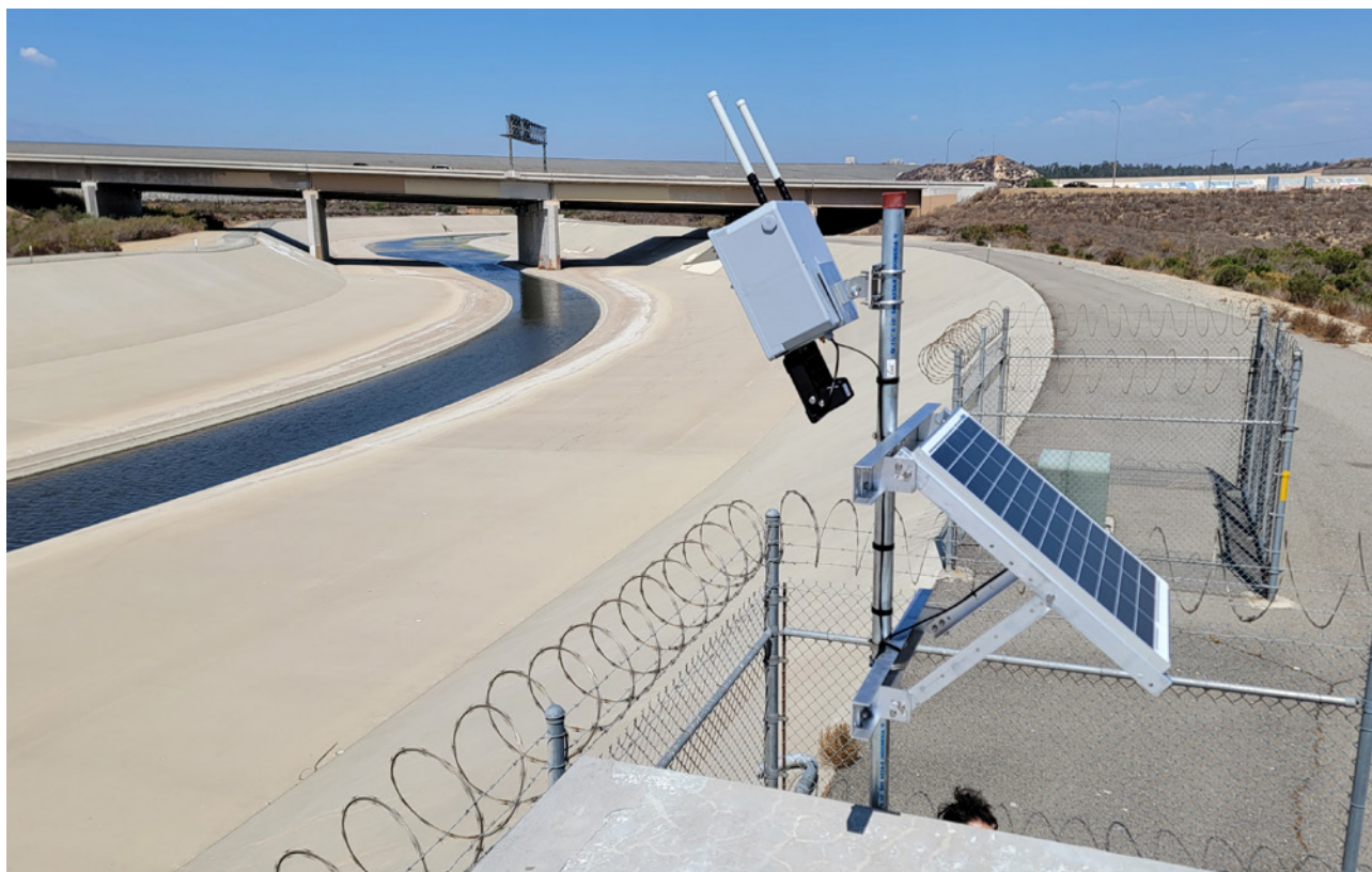
Figure 3: CVSG system installed at USGS gaging station 1107400, Santa Ana R BL Prado Dam, CA.
